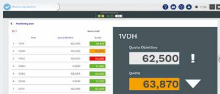
MDI (Memory Data Input) function for guided manual adjustment of axes.
