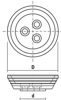
It mounts in place of the standard end cap to simplify the handling of heavy cutter stock
