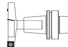
HW INSERT SPOILBOARD CUTTER INTEGRATED WITH HSK-63F
