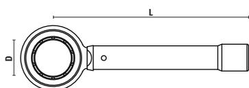
Dr. ① Collets as per drawing n. 1 must be tightened by setting the minimum torque value and rotating the handle counterclockwise.
