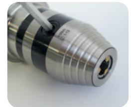
How to clamp the tool with key
