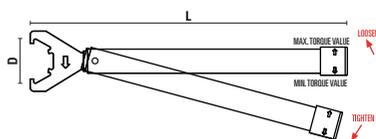
Dr. ① Collets as per drawing n. 1 must be tightened by setting the minimum torque value and rotating the handle counterclockwise.
